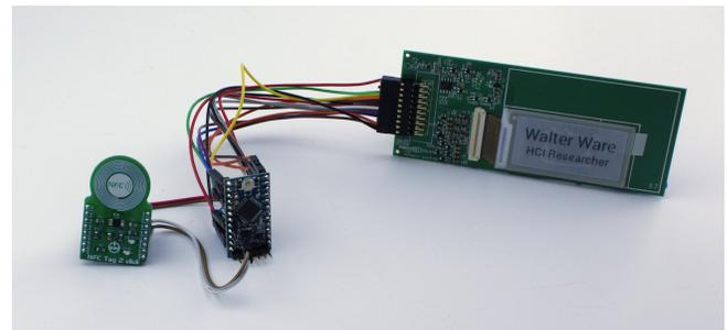
**Figure 3.** Our larger prototypes use an NFC Tag 2 Click breakout board, an Arduino Pro Mini microcontroller, and an e-ink display with EPD Extension Kit. While these components are relatively large and bulky, the size can be significantly reduced with custom hardware (see Figure 8).
