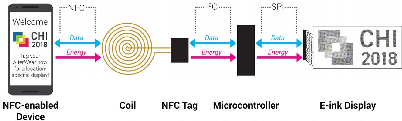
**Figure 4.** The AlterWear architecture includes an NFC tag, a microcontroller, and an e-ink display that are powered and updated through contact with an NFC-enabled device. When the device comes into contact with AlterWear, energy and data are transferred via NFC. The NFC tag then powers and transfers data via I2C to the connected microcontroller. Finally, the microcontroller powers and communicates with the e-ink display over SPI.
