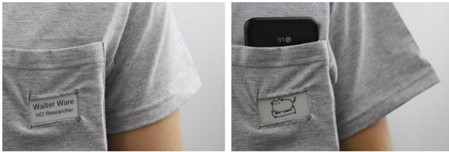
**Figure 5. Pocket tee prototype.** Left: name tag application. Right: when the user places their NFC-enabled phone in their pocket, the phone continuously powers the display, and a simple animation is displayed.
