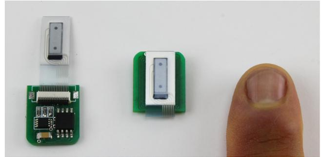
**Figure 8. The fingernail AlterWear design with custom circuitry and e-ink (Left) and folded over into a more compact fingernail form factor exposing the dynamically programmable e-ink dot pattern (Middle) next to an actual fingernail (Right).**
