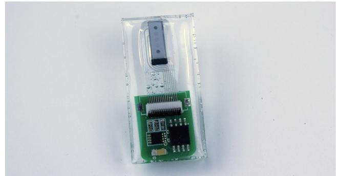
**Figure 12.** To demonstrate durability and longevity of AlterWear devices, we completely enclosed our fingernail prototype in resin. The prototype is durable, waterproof, and still entirely functional.
